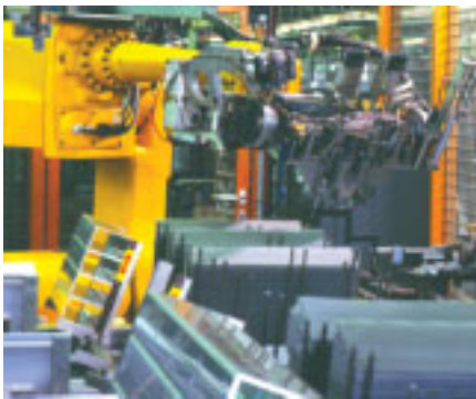
Robot for the assembly of cooling cores
